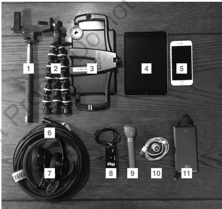
Photo 5.6 A typical mobile journalism go-bag contains the following: 1. selfie stick 2. mini tripod 3. iOgrapher filmmaking case 4. iPad Mini 5. iPhone 6. XLR cable 7. headphones 8. iRig Pre XLR adaptor 9. microphone 10. car charger 11. portable charger
